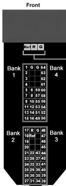
Pins for jumper connections.
