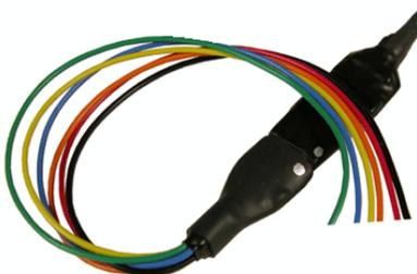
Available with flying leads. When connecting to the headstage, note that the silver dots marking channel 1 line up. The colors of the lead wires correspond to the headstage channels as shown in the table to the right.
