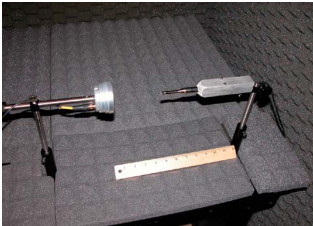
Figure 4 The sound chamber at TDT which is used for testing and calibrating speakers.
