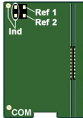
Connecting a jumper between the headstage reference pins and either the REF1 or REF2 pin connects the headstage reference to the desired probe reference [see table left for more information].
