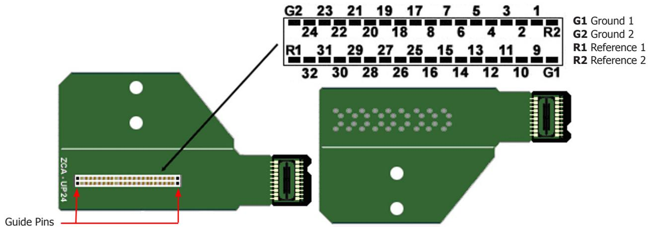
Pinouts are looking into the connector and reflect the preamplifier channels.
