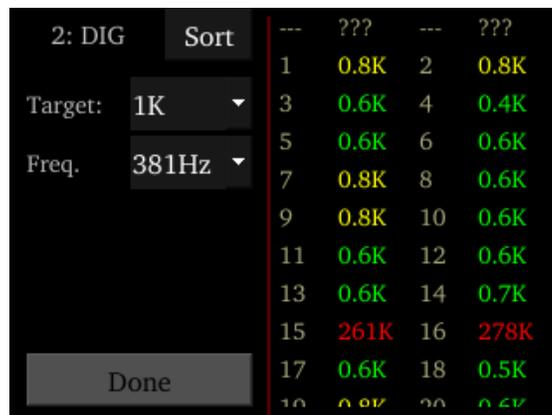
5. A limited set of channels is visible at any one time. Swipe vertically on the interface to scroll the visible channels or touch the Sort button to sort the list by channel number or by impedance value.
