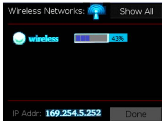
The wireless icon
