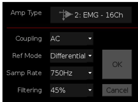
Each Amp Type includes preset values for each setting. The Configuration Options screen enables users to modify these settings.
