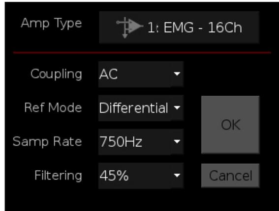
6. Make any desired changes to the default settings then touch the **OK** button to save the selections and return to the Main Configuration screen.
