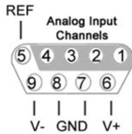
A 4-Channel connector is found only on models shipped before January 2002. **Note:** Pins 7 & 8, tied together.
