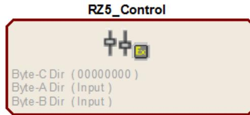
Double-click the macro to access the settings on the Digital I/O tab. The RZ5\_Control macro also offers a Direction Control Mode parameter that enables the macro inputs and allows the user to control data direction dynamically. For more information on using the RZ5\_Control macro see the help provided in the macro's properties dialog box. For more information on addressing and “Digital I/O” see the *RPvdsEx Manual*.
