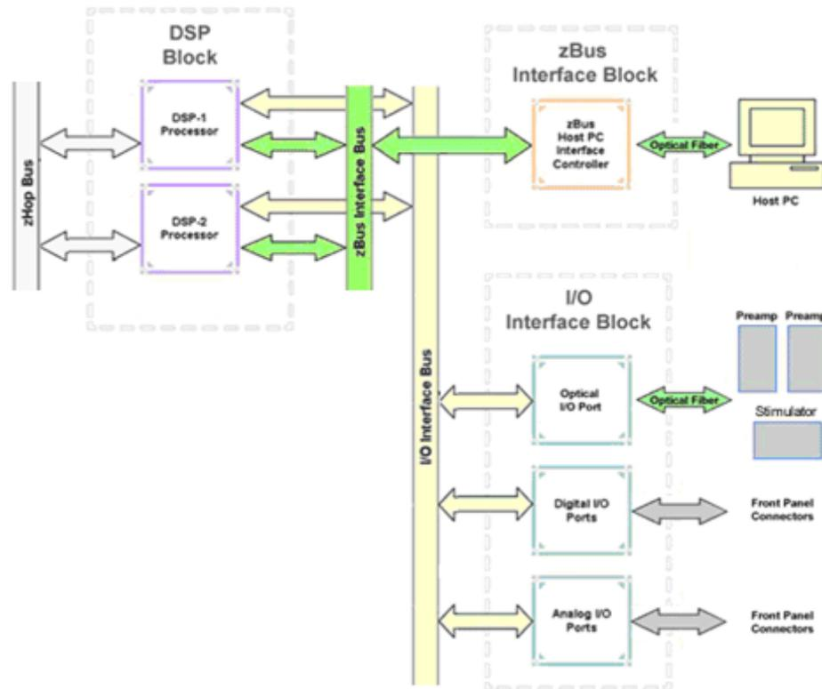
As shown in the diagram above, the RZ5 architecture consists of three functional blocks:
