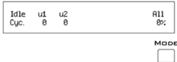
The front panel display screen reports detailed information about the status of the system. The display includes two lines. The top line reports the system mode, Run!, Idle, or Reset, and displays heading labels for the second line. The second line reports the user's choice of status indicators for each DSP followed by an aggregate value.
