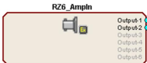
Input from the preamplifier fiber optic port is accessed using the RZ6\_Ampln macro.
