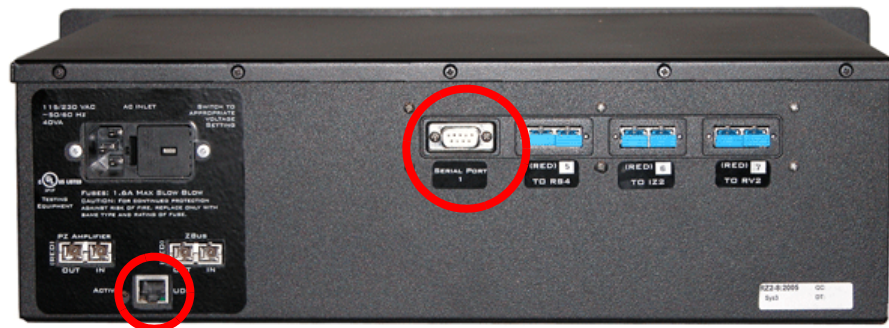
RZ2 Processor Back side with RZ-UDP Installed
