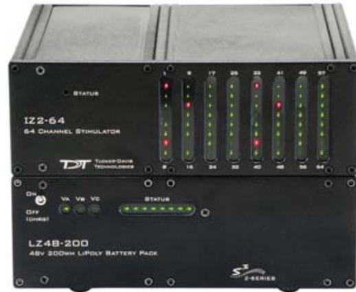
**Power and Communication.** The LZ48 Battery Packs use multiple Lithium Polymer [LiPoly] batteries to power both the stimulation and the IZ2 stimulator logic circuitry. A 24 Volt battery charger with 2.7 A of current capacity is included with the stimulator and can be connected via the connector on the LZ48's back panel.
